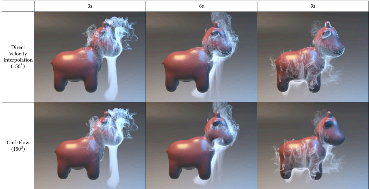
Fig. 21. A Smoke Plume Simulation with A Solid Shaped like A Calf. In the direct velocity interpolation case, a large number of particles erroneously collide with the solid and are then frozen, especially around the ears and underside of the head; with Curl-Flow, more particles flow smoothly over and around the object's surface and since more smoke remains active it is denser and brighter (middle column, above the face, and see video).
