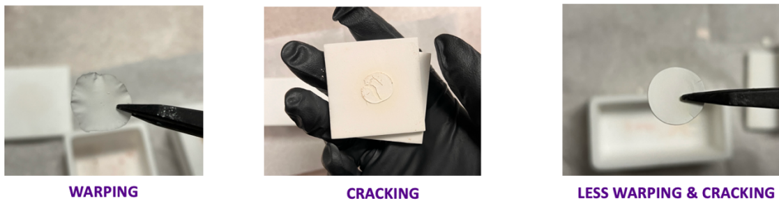
Figure A7: Optical images of warping and cracking LLZO solid electrolyte sintering challenges. A flatter ceramic is observed after implementing a pressing and cutting step to pack solid particles together and cutting thinner edges out.
