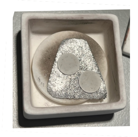
Figure A8: Optical image of MgO sandwich sintering technique within the 12mL MgO crucible.
