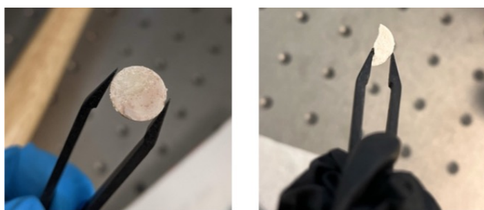
Figure A2: Optical images of sintered LLZTO bulk pellet with uneven sintering (left) and broken brittle bulk pellet (right).
