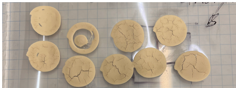
Figure A4: Optical images printed ceramic electrolytes cracked during drying.
