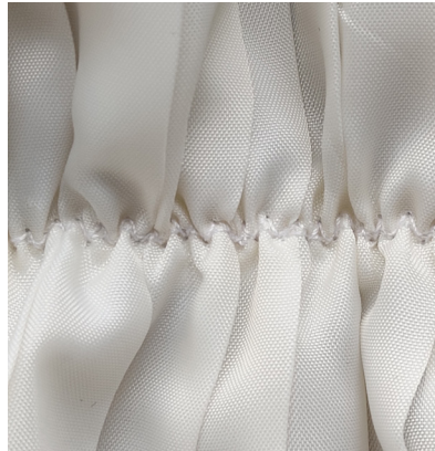
b. The elastic is sewn to the cuff using a zig-zag stitch for added reinforcement and flexibility rather than a straight stitch.
