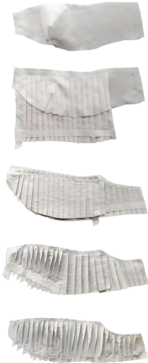
Fig. 4.109 Process of sewing the twisted knife pleats for the bust of the dress.
