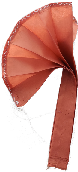
Fig. 4.106 Hemming the edge of a pleated piece of fabric after it was ironed expands the pleat along the seam. This is a way to show off the existence of the pleat without the use of movement to reveal itself.
