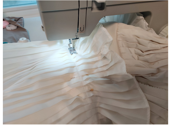
b. Sew waist pleats panel to the dress, aligning the centerline of the waist pleats to the waist of the under-dress and front skirt.
