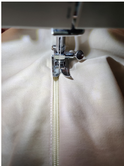
d. Sew another straight stitch to lay the fabric flat against the zipper. This pulls the fabric away from the zipper to prevent the fabric from getting caught while using the zipper.
