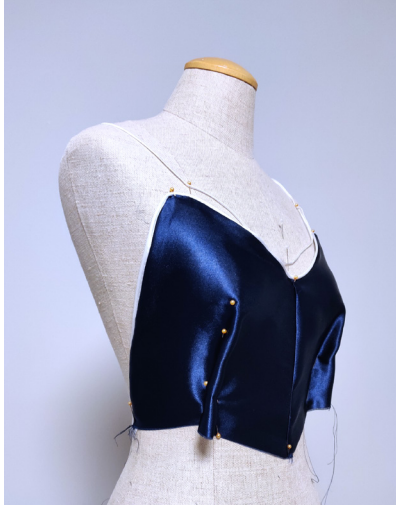
Fig. 4.43 Pinning the bodice to a mannequin to map out the darts beneath the bust.
