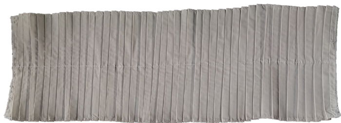
Fig. 4.120 Collar is made of one panel of knife pleats with heavyweight polyester.
