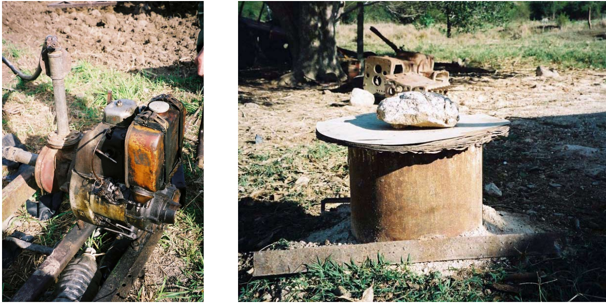
Figure 5.1: A water pump that has been modified to run on manual power when gasoline is unavailable (left); a well waits for the installation of a power source - the farmer hopes for a windmill - in order to become functional (right).
