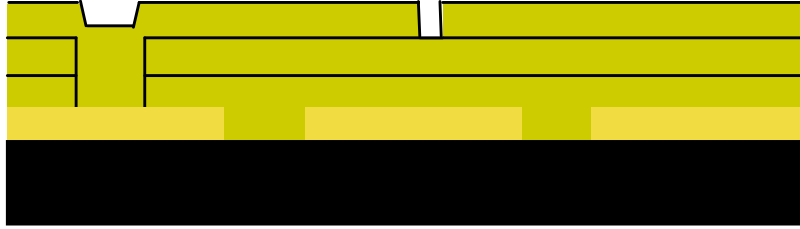
Figure 5.25: Cross section of three layers of polyimide. Etching the first two layers and then coating and etching the third layer ensures no holes will span the full depth of the polyimide.
