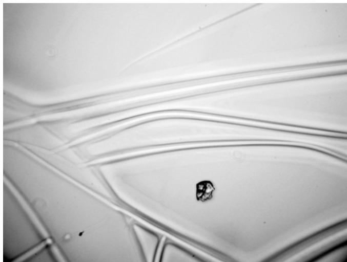
Figure 5: Microscope image of the surface of polyimide PI 2611 after coating with a second layer before curing the first layer. Unlike PI 2562, PI 2611 must be fully cured before applying additional layers.
