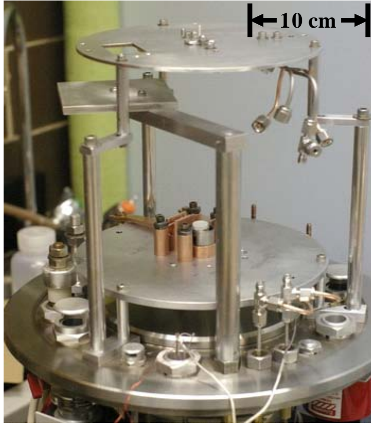
Figure 5.3: Modified Edwards evaporator. This is located in the Department of Physics senior undergraduate laboratory area.
