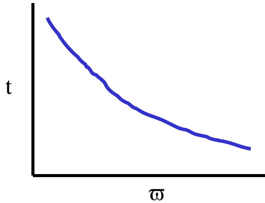
Figure 3.1: Typical spin curve plotting spun thickness vs. spin speed [48].
