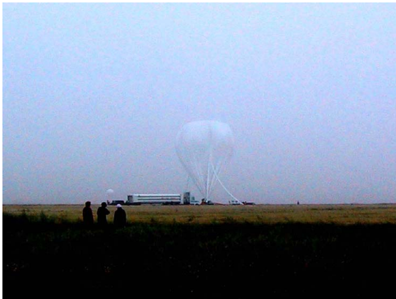
Figure 2.3 MANTRA 2004 balloon was launched on September 1 st , 2004. It contains 330208 m 3 (11.8 million cubic feet) of helium gas and carried 13 scientific instruments with a total weight of 658 kg (1450 lb) to the float altitude of about 37 km. Figure was downloaded from http://www.atmosp.physics.utoronto.ca/MANTRA .
