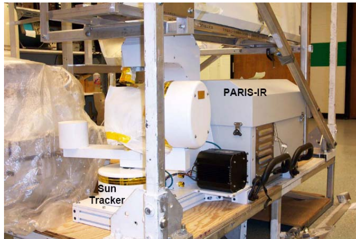
Figure 4.4 PARIS-IR and the ABB-Bomem sun tracker on the gondola of the MANTRA 2004 balloon during mechanical tests.
