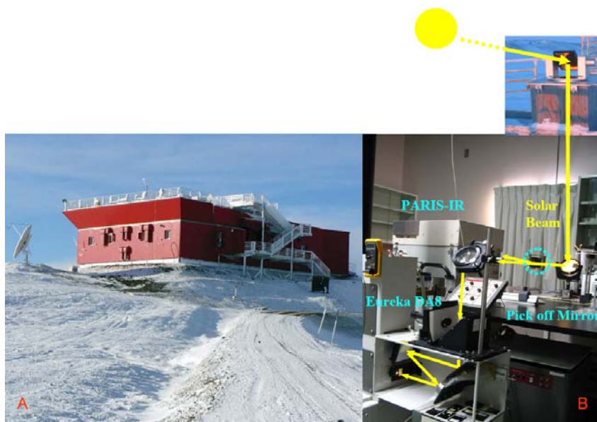
Figure 2.7 Overview of the PEARL and two FTSS in the Eureka 2006 campaign. (A) PEARL located at Eureka, Nunavut Canada; (B) the ABB-Bomem DA8 spectrometer and PARIS-IR simultaneously observing the Arctic atmosphere in PEARL from February 21 st to March 8 th , 2006.
