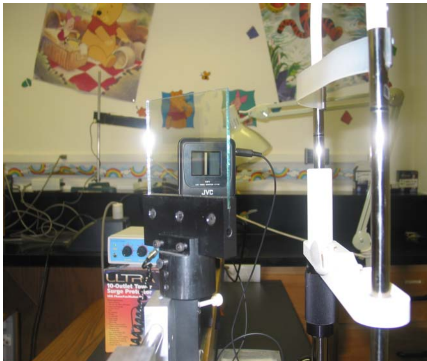
Figure 4.1 showing DoG target projected onto the semisilvered mirror from the LCD monitor at 0.4m
