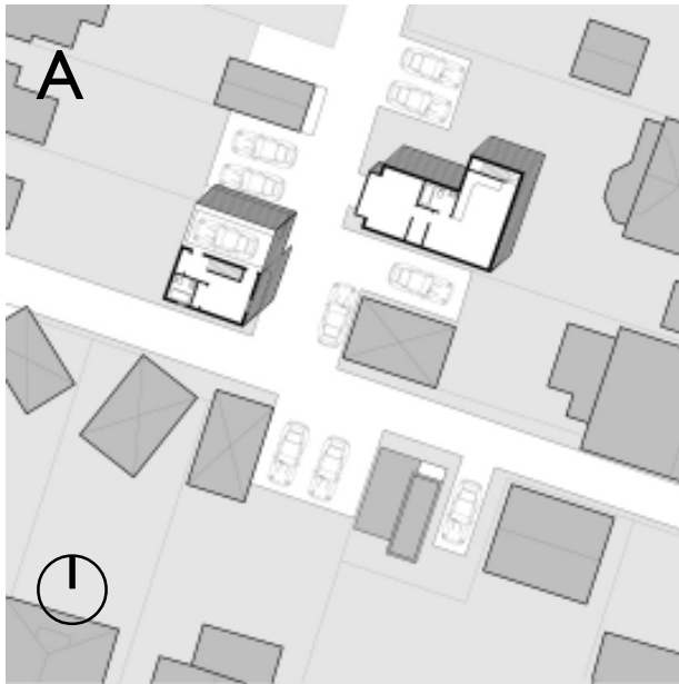
5.27 (Location indicated on map 5.26 with “A”) Piloti House and Above-Shop infill house in low-density infill scenario of St. Clair neighbourhood context, including afternoon shadow study (September 21st).
