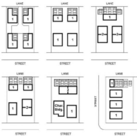
2.17 Vancouver’s R-10 guidelines allow for multiple residential buildings on a single lot, as well as lot assembly. Diagram shows possible configurations for two lots which have been assembled.
