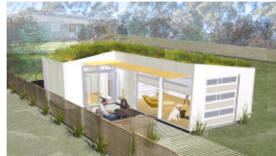
2.37 ADU prototype utilizes SIPs construction, a trombe wall and greywater storage and re-use. Design by CSS Architecture.
