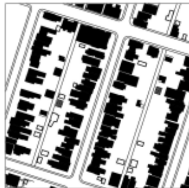
5.46 Figure-ground comparison of target laneway infill scenarios for three neighbourhood test cases. From these studies, maximum targeted infill density from laneway housing is approximately 30 households per hectare.
