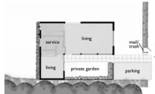
2.38 Plan and rendering for ADU prototype with prefabricated wall panels and a green roof. Design by Peterson Architects.
