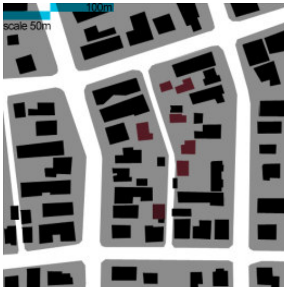
2.40 Figure-ground diagram of a typical block in Santa Cruz with potential for ADU infill.
