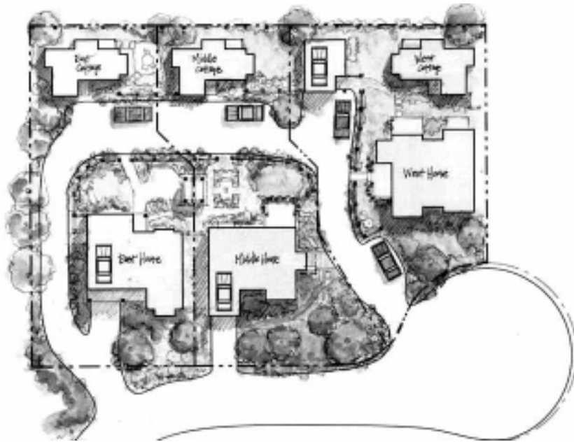
2.30 Site plan of 'Backyard Neighbours' pocket development in Langley, Washington, which employs a doubling in housing density through the Cottage House Development zoning.
