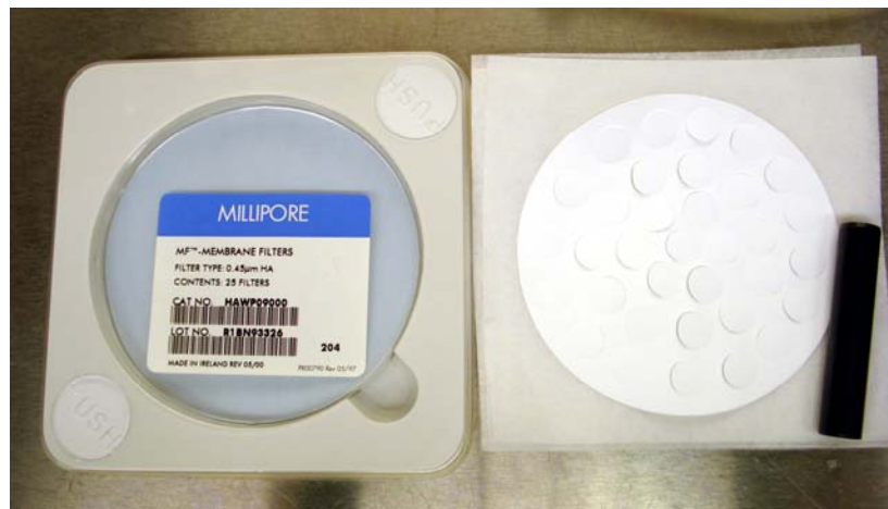
Figure 3-12: Large Millipore MF™ membrane filters were used to make discs of 10mm diameter for impression cytology
