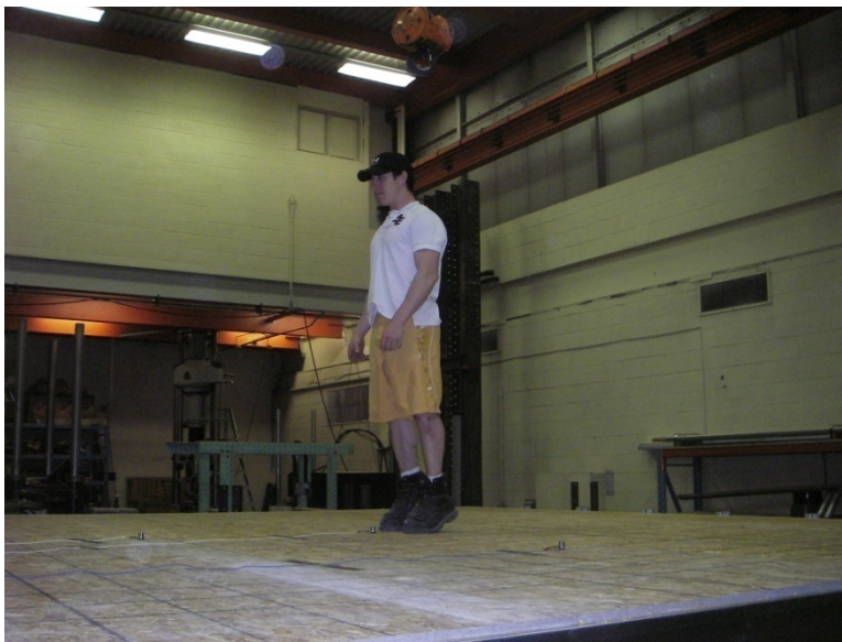
Figure 3-6: Heel Drop Test
