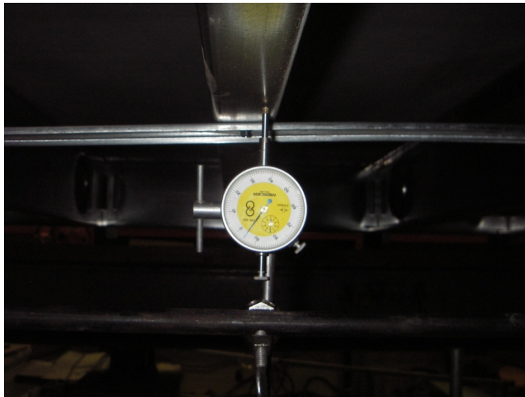
Figure 3-7: Joist Deflection Measurement
