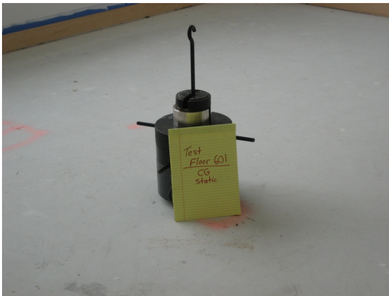
Figure 3-9: 1 kN Load from Static Test (Field)
