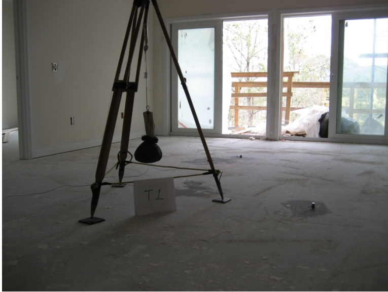
Figure 3-5: Sandbag Drop Test (Field)
