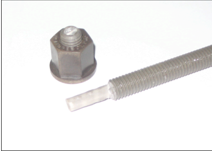
Figure 4.9 - Slip Failure of the Fiberbolt Under Direct Tension
