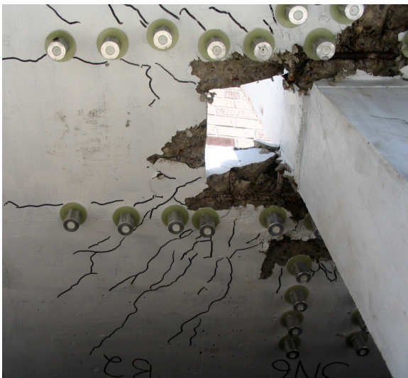
Figure 5.14 - Crack Pattern, Tension Side of Slab, SN6
