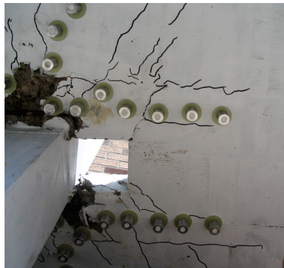
Figure 5.14 - Crack Pattern, Tension Side of Slab, SN6
