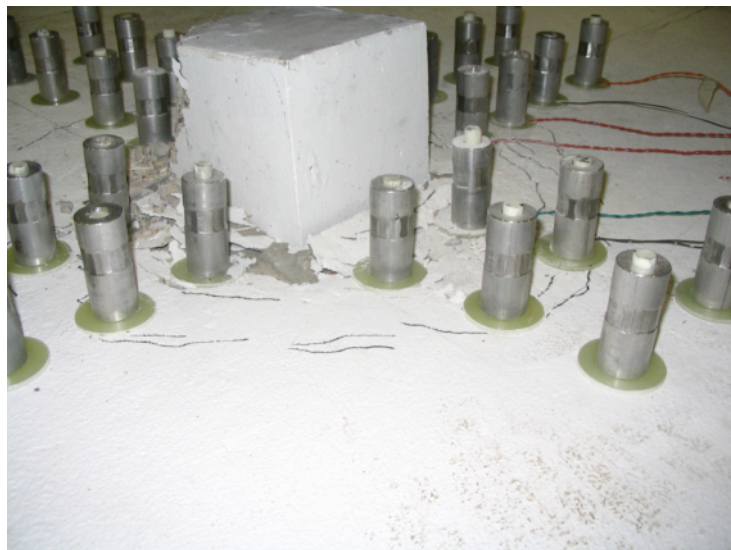
Figure 4.6 - ComBAR Type Shear Bolts during testing
