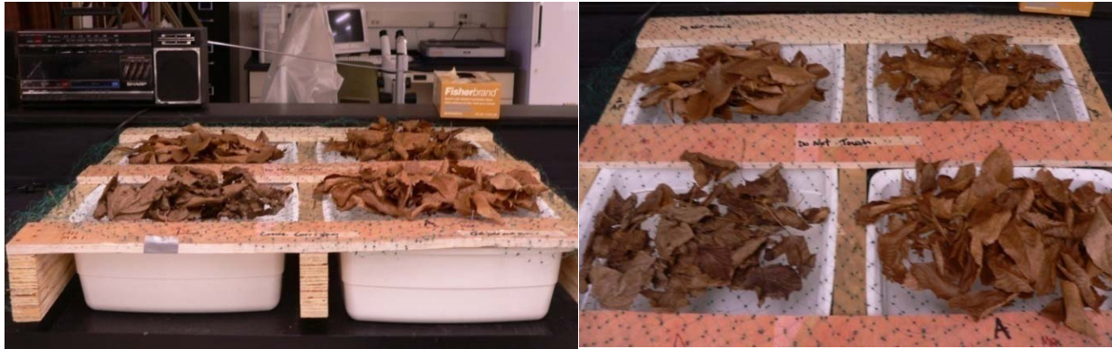
Figure 3.3: Experimental set-up of leaf litter leaching with exposure to 0 (Ctrl), 30 (L), 60 (M) and 100 mm (H) to evaluate changes in litter nutrient content and DOC, DON and DIN or the leachate. Photo taken by Cassie Corrigan.
