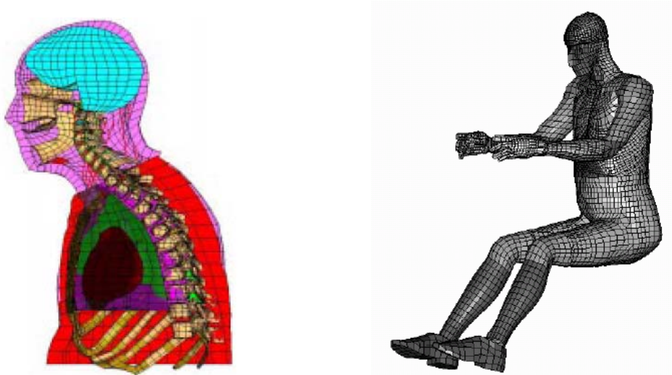
Figure 2.20 Numerical Human Body Models (a) Sagittal Section of Humos Upper Body (HUMOS, 2001) (b) Ford Motor Company Human Body Finite Element Model (Ruan et al., 2003)
