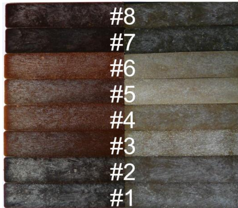
Figure 4-27 Bars from Run # 1 – 8 before (left) and after (right) 161 days immersion in water.
