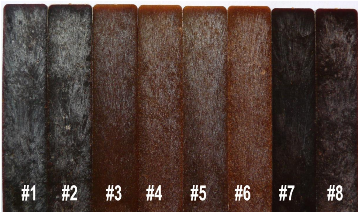
Figure 4-20 Biocomposite bars from Run # 1 - 8 (left to right) after injection moulding.
