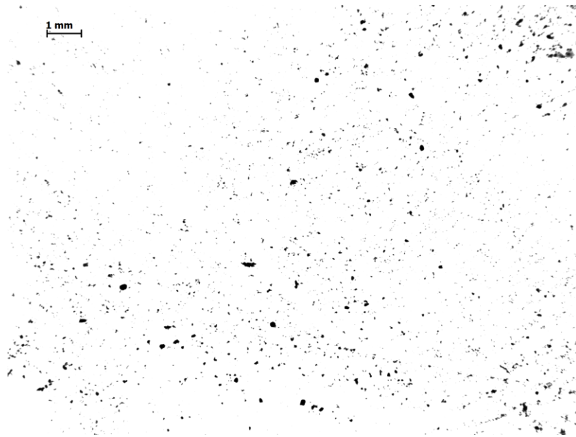
Figure 5-6 Representative image of particle size analysis of soy flour (Ford).
