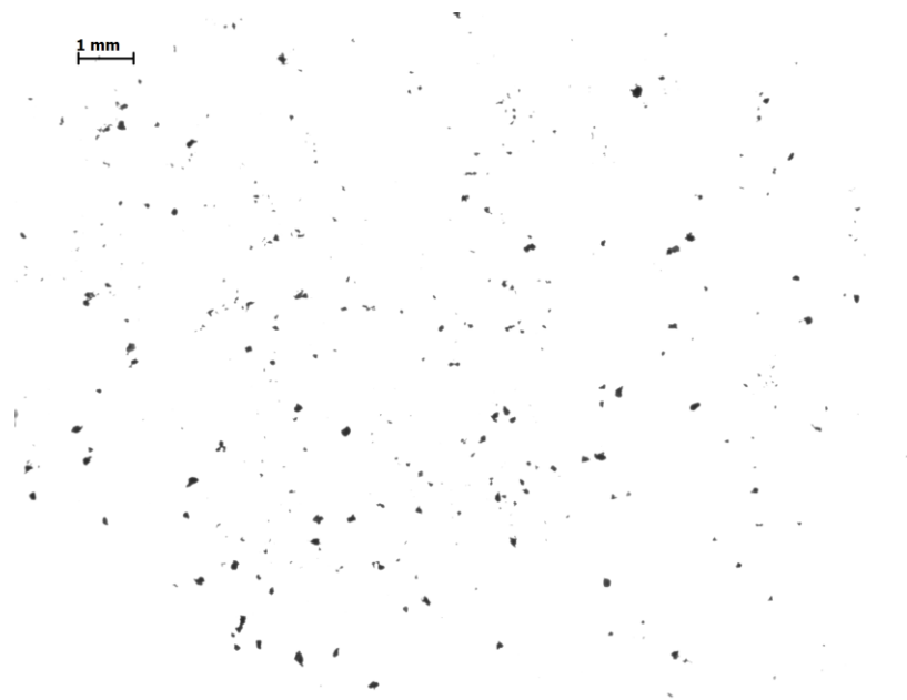
Figure 5-5 Representative image of particle size analysis of IS_{NaCl} .
