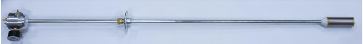
Figure 3-7 Overall view of the dipper probe structure.
