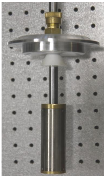
Figure 3-6 (Left) the closed sub-module is shown before installing it in the helium Dewar. (Right) The opened sub-module with the SNSPD package and the thermally anchored semi-rigid coax cable.
