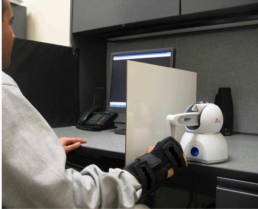
Figure 3.5: The subject grasps the end-effector of the PHANToM TM Omni and rotate his hand about his elbow.
