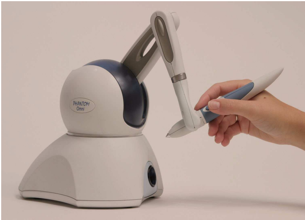
Figure 3.1: The PHANTOM TM Omni device made by SensAble Technologies Inc. [69].
