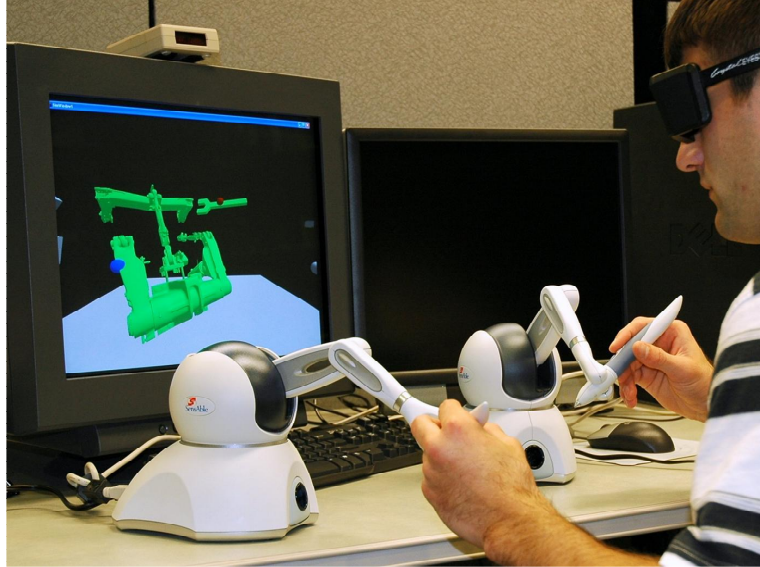
Figure 2.1: Computer-aided assembly using force feedback haptic devices [16].
