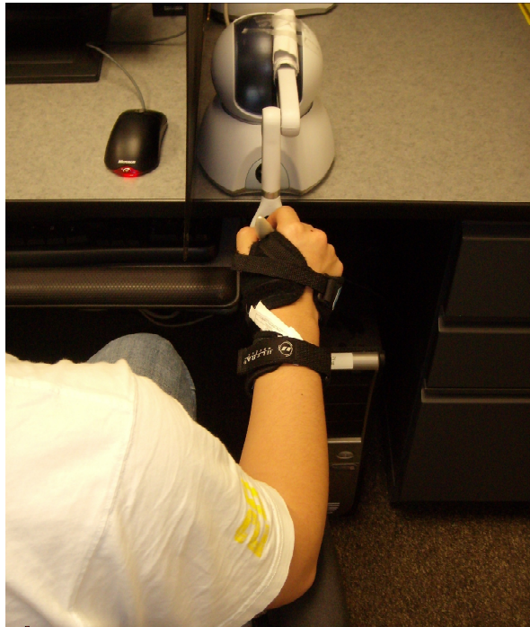
Figure 4.2: The subject grasps the device end-effector while he places his right elbow on a side support.
