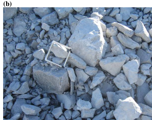
Figure 3-3: Typical instrumentation face (a) entire face; and (b) instrumentation face sample area. Square scale in (a) is 0.5 m by 0.5 m and highlighted yellow with arrow for clarity; white square scale in (b) is 0.5 m by 0.5 m.
