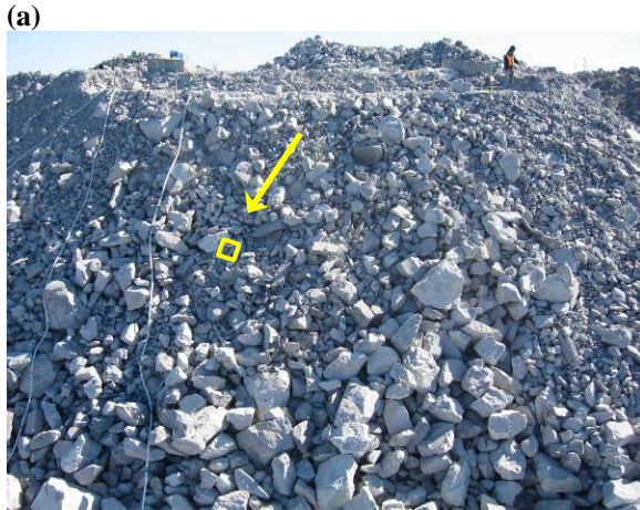
Figure 3-3: Typical instrumentation face (a) entire face; and (b) instrumentation face sample area. Square scale in (a) is 0.5 m by 0.5 m and highlighted yellow with arrow for clarity; white square scale in (b) is 0.5 m by 0.5 m.
