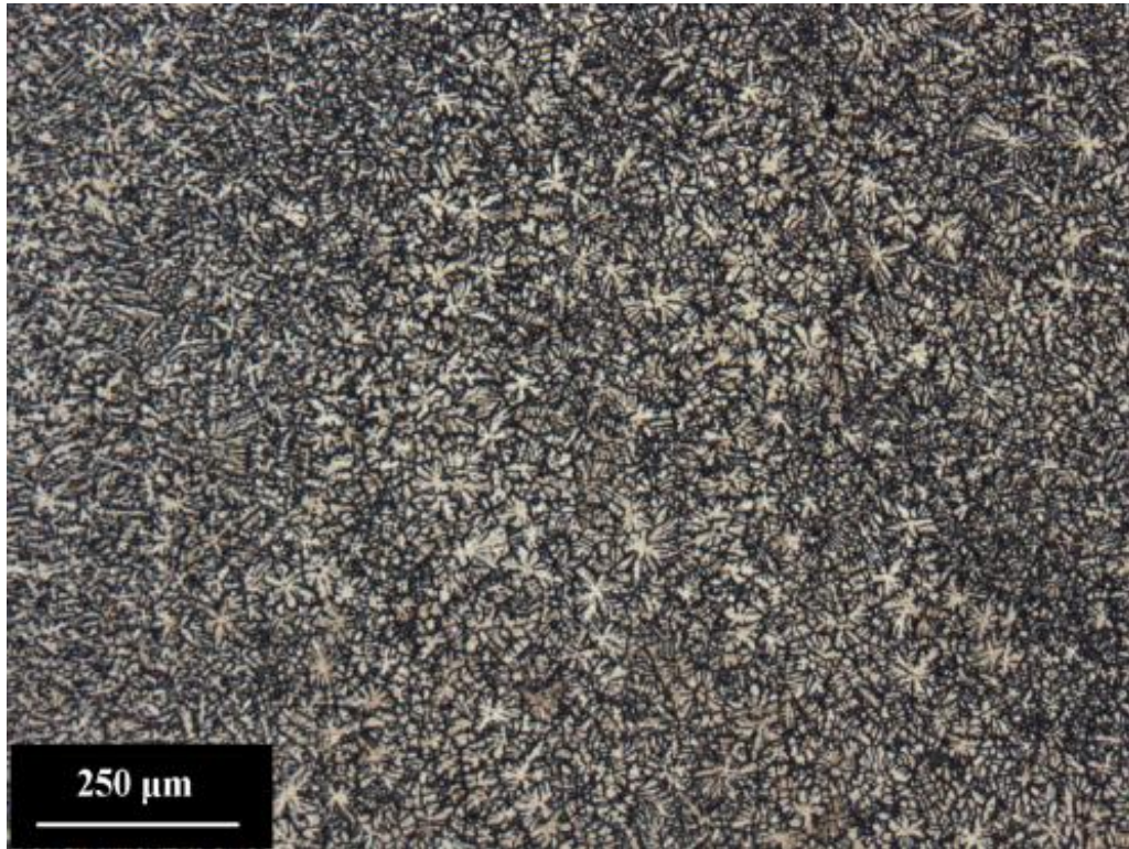
Figure 4-8: Representative equiaxed-dendritic solidification microstructure found in the center of the diode laser welds where the solidification growth rate was high.
