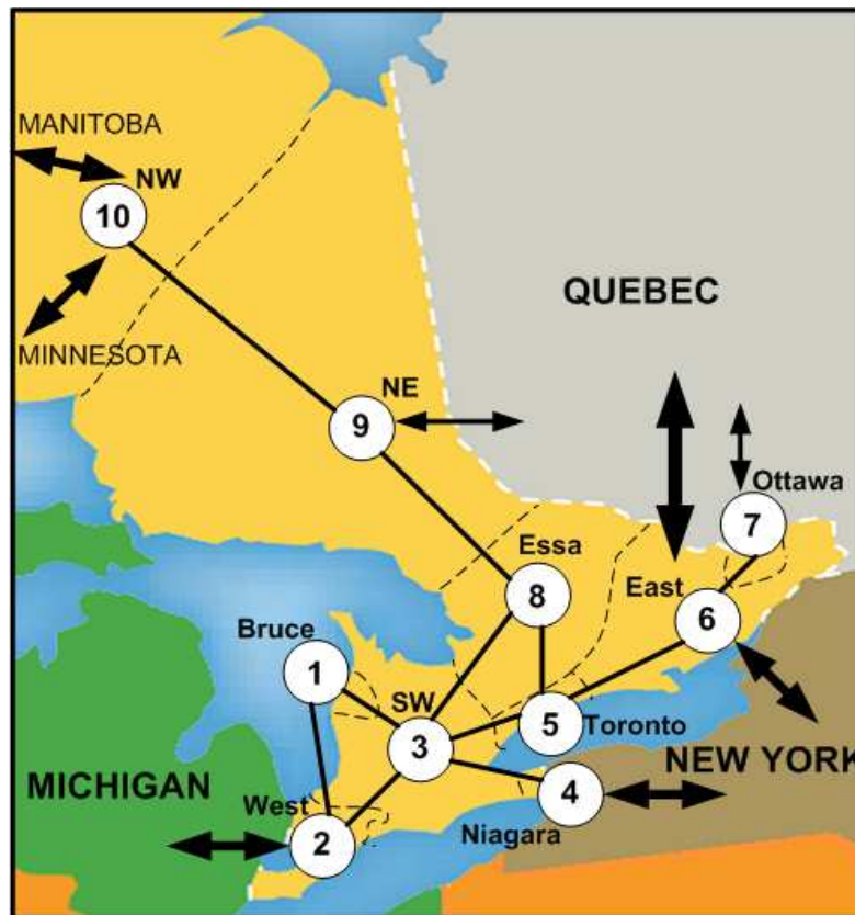
Figure 4.1: Simplified model of Ontario's grid.
