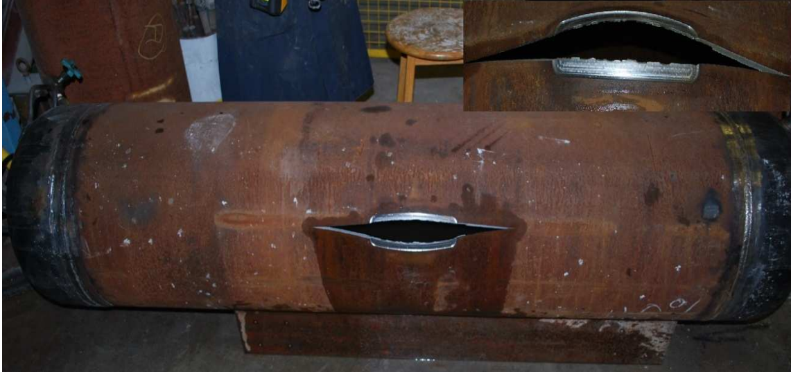
Figure 3.2 Burst Test of The 61%WT Corroded Pipe [9]
