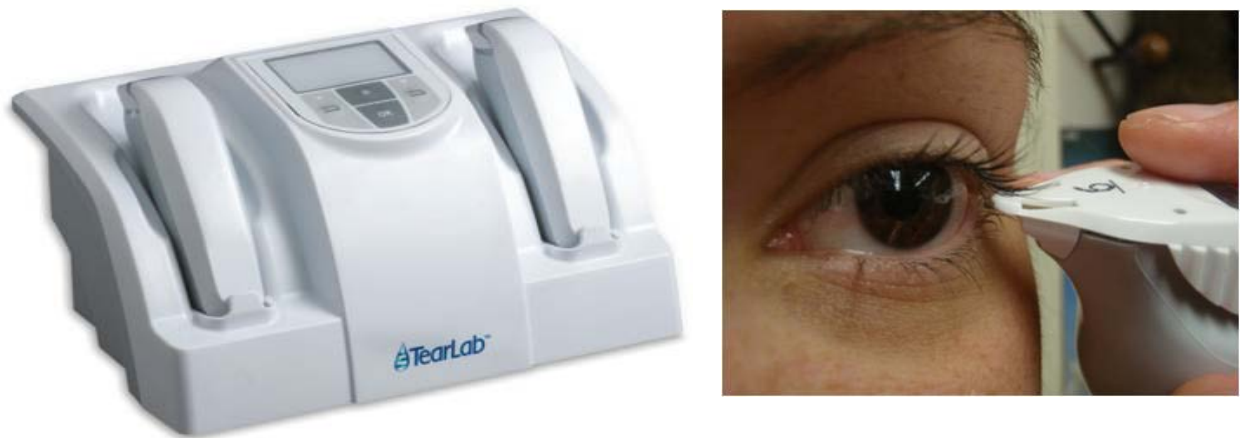
Figure 1-4. TearLab™ unit and collection technique with the handheld pen and chip card.
