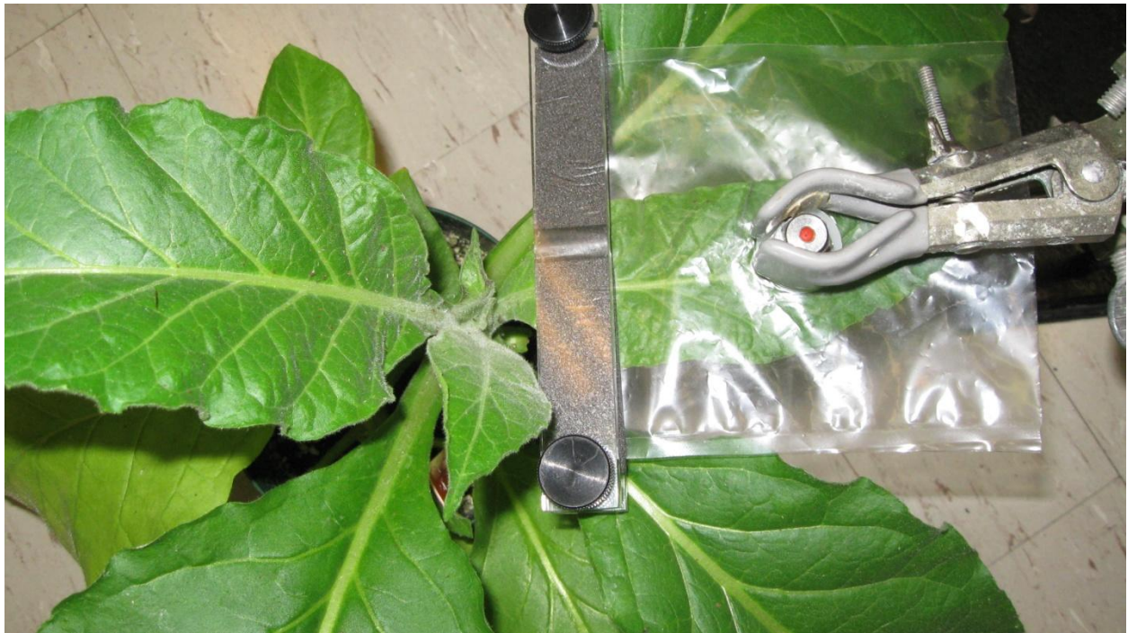
Figure 5. A young transgenic tobacco leaf in a Tedler bag, with the top of the bag closed with a clamp. The bag enclosure method was employed to collect foliar in vivo emissions of C 2 H 4 , CH 3 Cl, and CH 3 Br.
