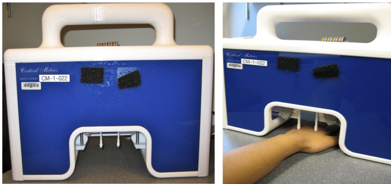
Figure 2.1: Cortical Metrics device pictured alone and pictured with a subject's hand dorsum under probes.
