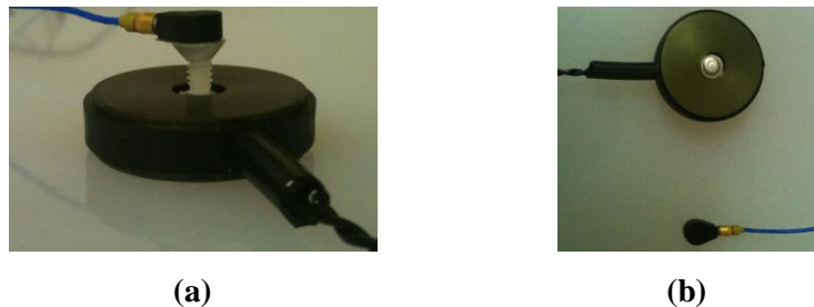
Figure 29: (a) Accelerometer attached to the contactor using a lightweight (0.5 gr) plastic screw, (b) accelerometer attached to the surface of the gel, 3 cm away from the external boundary of the tactor.
