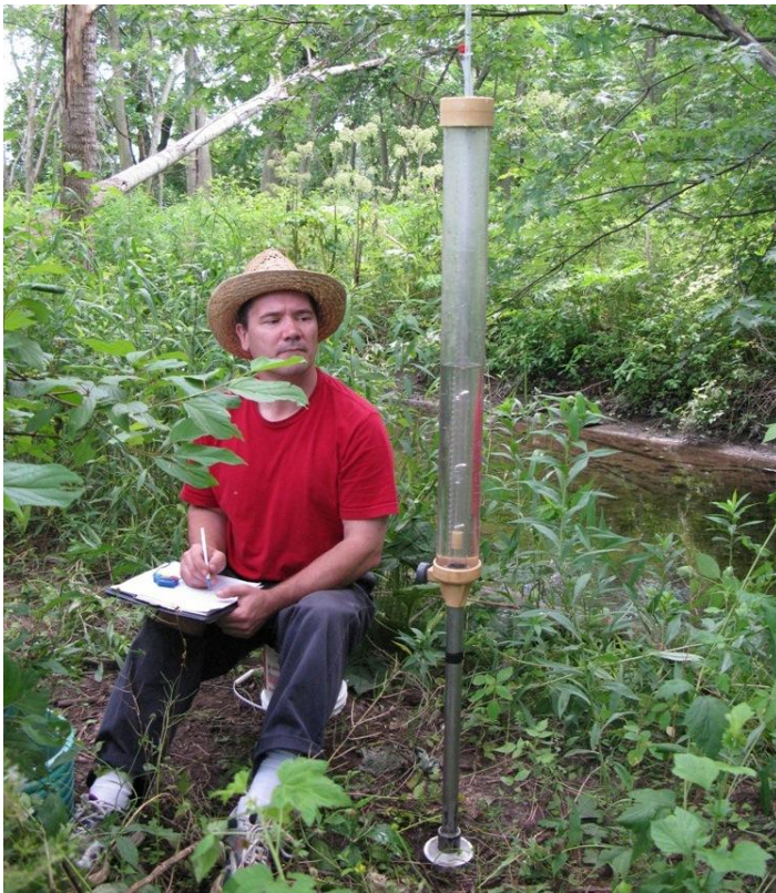
Figure 2.8. Determining hydraulic conductivity in the rehabilitated riparian zone with a Guelph pressure infiltrometer.
