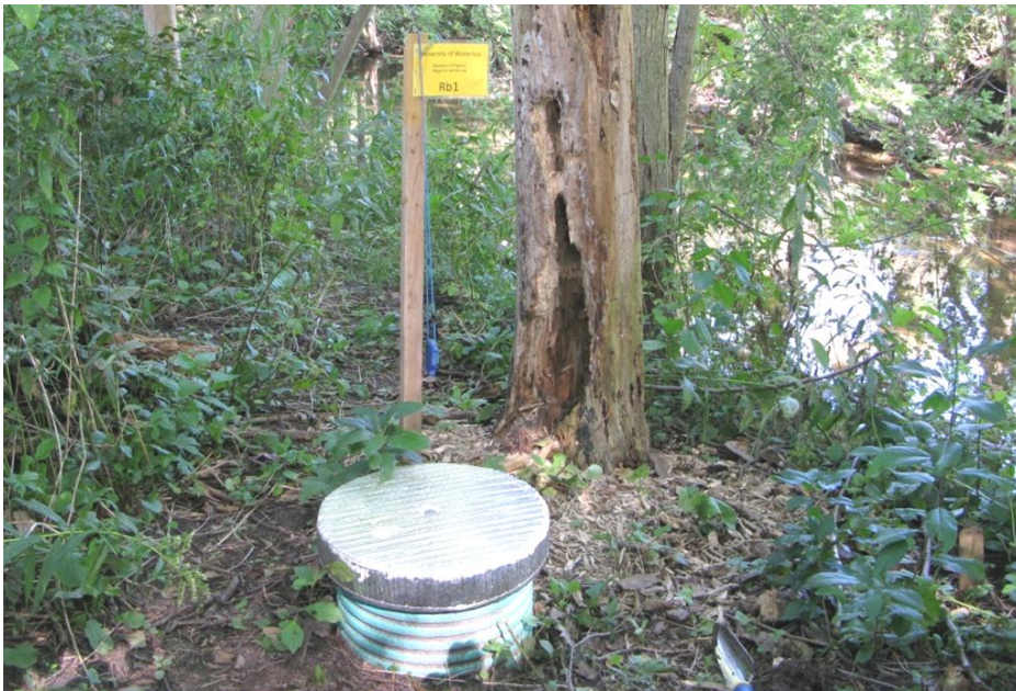
Figure 2.9. Chamber for measuring soil CO 2 with cap on located in the rehabilitated riparian zone along Washington Creek, Ontario.
