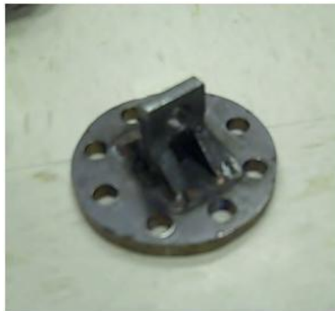
Figure 3.9: Part designed to restrict internal/ external rotation.
