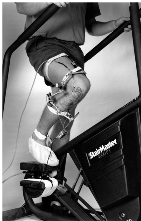
Figure 2.2: Test setup for measuring ACL strain during StairMaster activity (Fleming BC, 1999).
