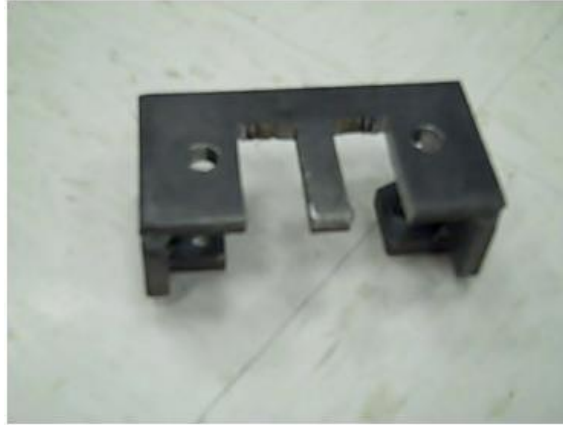
Figure 3.8: New part designed to restrict internal/ external rotation.
