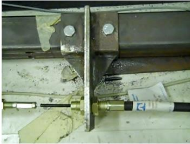
Figure 3.11: Top view of redesigned calf muscle actuator bracket.
