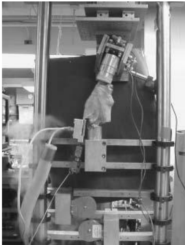
Figure 2.5: Cadaver knee potted in a jig flexed at 20 degrees (DeMorat G, 2004).
