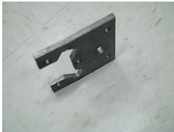
Figure 3.7: Side profile of modified plate at ankle joint.
