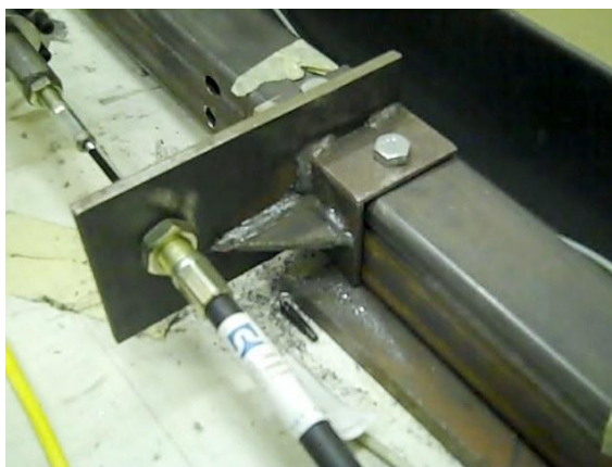
Figure 3.10: Redesigned calf muscle actuator bracket.
