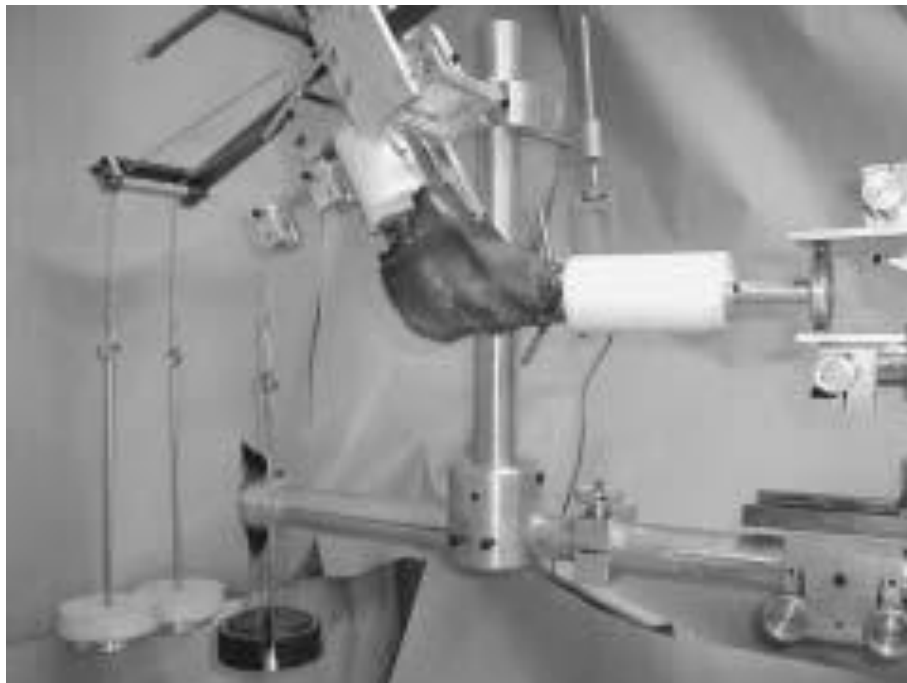
Figure 2.6: Testing apparatus applies muscle loads as the knee is passively extended under various tibial loading conditions. The femur (shown at left) is extended relative to the tibia, which is maintained in a level position throughout the range of motion. The roller at the end of the potted tibia (shown at right) allows unrestrained tibial rotation and varus-valgus angulation (Markolf KL, 2004).
