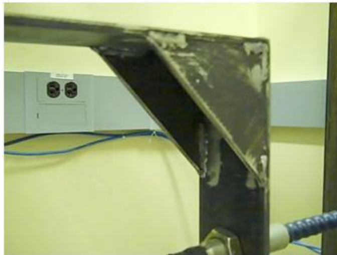
Figure 3.5: Triangular pieces used to reinforce hip component.
