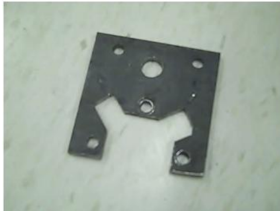
Figure 3.6: Modified steel plate at ankle joint.
