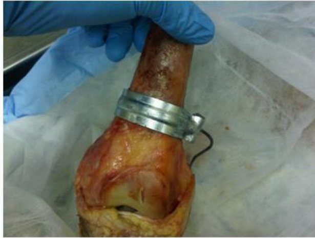
Figure 4.17: Front profile of knee with rigid steel wrap used for calf muscle insertion site.
