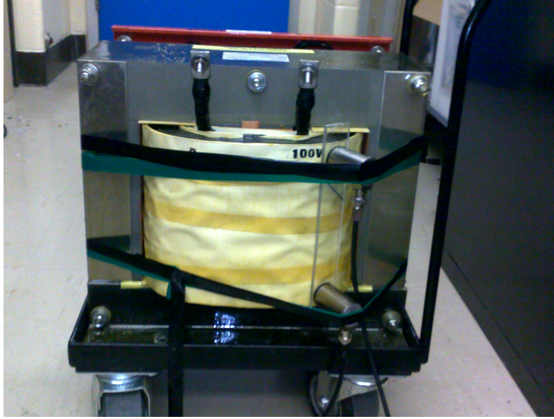
Figure 5.1: 100/10,000 V, 10 kVA resin dry-type transformer
