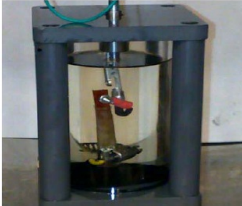
Figure 6.9: Transformer paper insulation test sample
