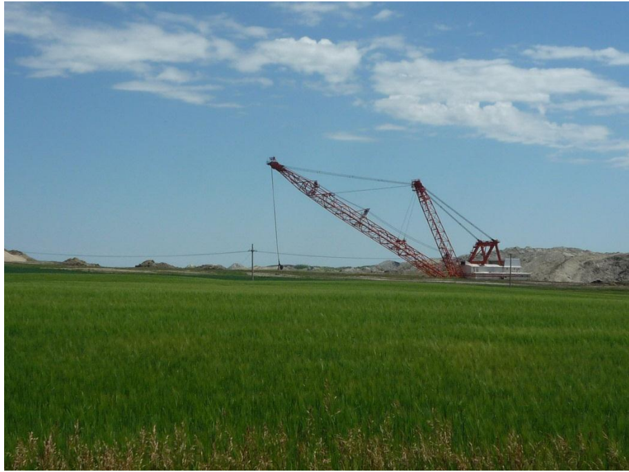
Figure 29 Largest Dragline in North America
