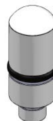
FIGURE 7-1: THE FORM-FITTING PISTON TO HOLD THE CONTACT LENSES. A CIRCULAR RING IS FITTED OVERTOP THE PISTON TO KEEP THE CONTACT LENS IN PLACE DURING CYCLING
