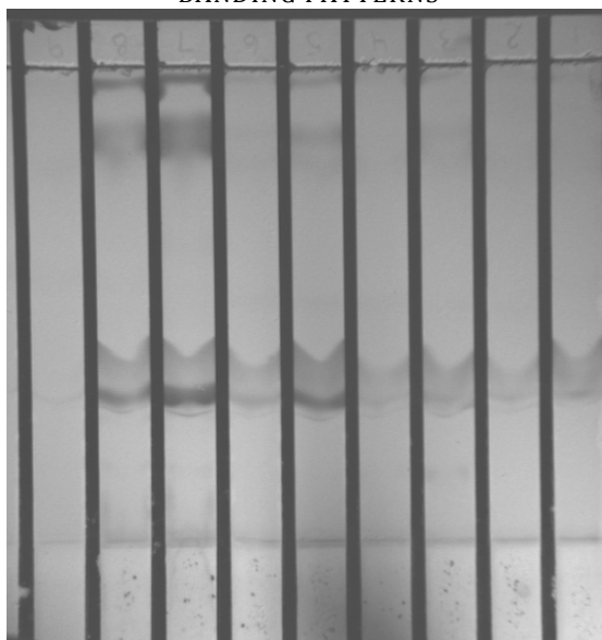
FIGURE 1-13: A SAMPLE TLC PLATE CHARRED WITH SULPHURIC ACID TO VISUALIZE LIPID BANDING PATTERNS
