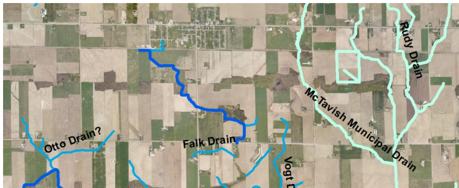
Figure 6-5: Fragment of projected drainage layer. Different blue shades correspond to different types of drainage channels.
