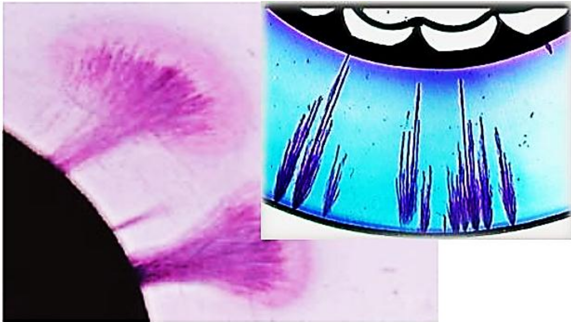
Figure 2.3: Accelerated growth of water trees from the conductor shield (left) and insulation shield (right) due to water-soluble ionic impurities [77]
