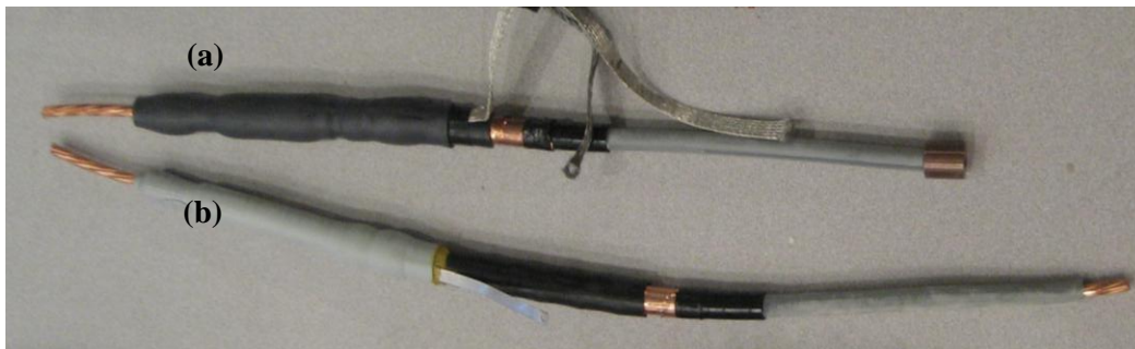
Figure 3.1: Cable termination samples that are considered in this study: (a) Type-II and (b) Type-I
