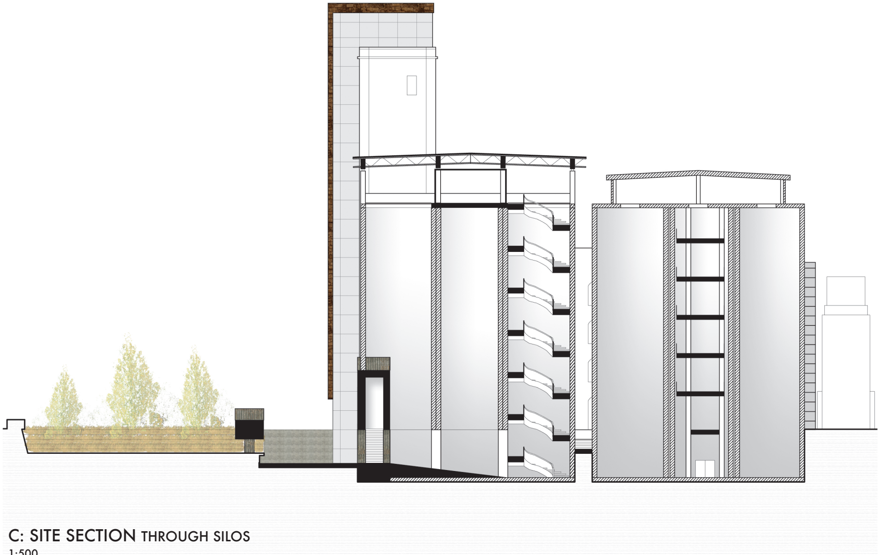
fig.3.2.9 Section C cutting through both silo complexes, revealing the circulation in both. The concrete silos use a lift to provide access for cleaning and maintenance.
