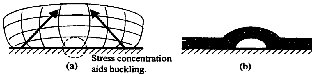
Figure 5.2: a) Qualitative cross-sectional portrait of a thin film with tensile stress. b) Catastrophic buckling failure from tensile film stress.
