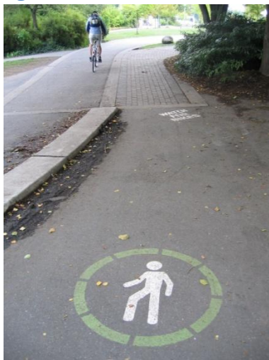
Fig. 66: Divided and marked trails help to keep pedestrian and cyclist traffic separate
