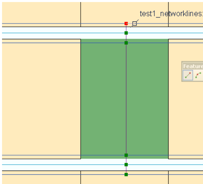
Fig. F.13: A trail extending across the road to connect with the closest ATN segment on the other side (here, a sidewalk)
