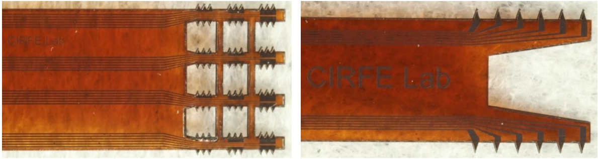
Figure 6-28. Flexible interconnect cables, Top: Single shaft electrode, Bottom left: Quad shaft electrode, Bottom right: Double shaft electrode carrier wafer
