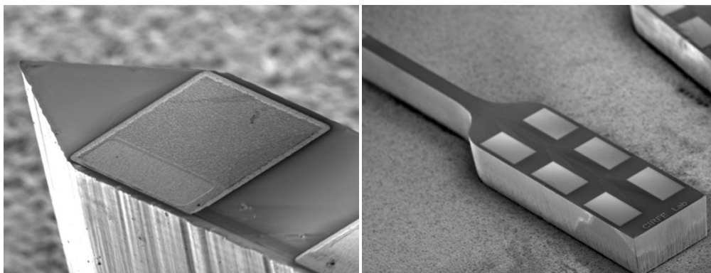
Figure 6-14. Double metallization layer stimulation electrode: SEM pictures for the electrode shaft demonstrating stimulation pads, vias and routing tracks
