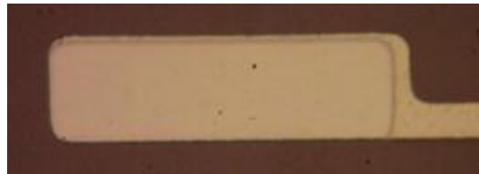
Figure 6-11. Modified via patterned using RIE in dielectric-2
