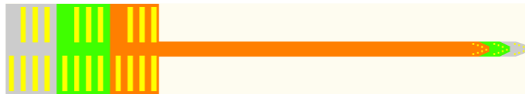
Figure 3-27. Multi-composite layer electrode, Layout A: 7 pads per layer
