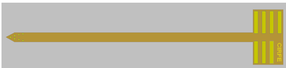
Figure 3-3. Basic simple recording electrode layout with 7 pads (Layout B)
