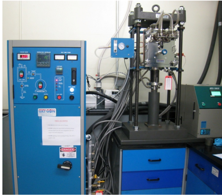
Figure 3.8 Hot pressing instrument of high temperature vacuum furnace system with 30 ton press capability by Oxy-Gon industries.
