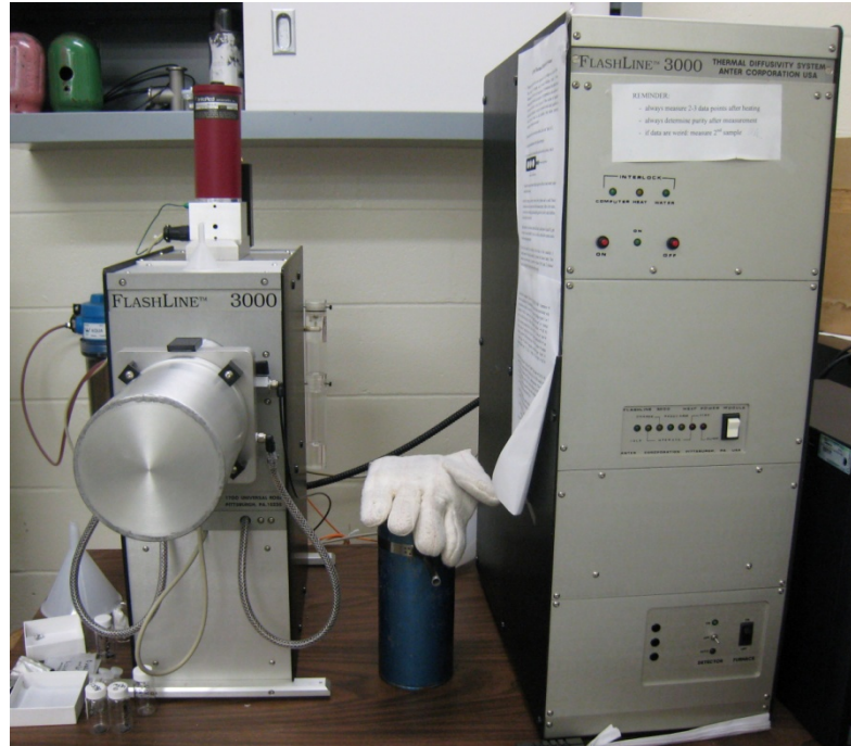
Figure 3.10 Flash Line 3000 thermal diffusivity system under argon (ANTER Corporation, viz).
