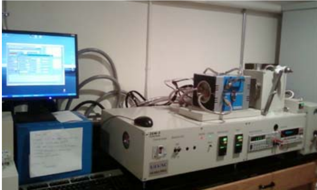
Figure 3.7 ULVAC-RICO ZEM-3 for the Seebeck coefficient and the electrical conductivity measurements.
