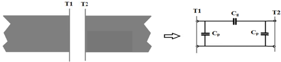
Figure 4-1: A microstrip gap and equivalent circuit model
