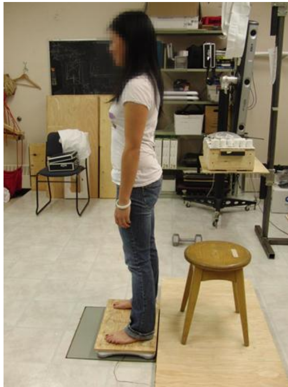
Figure 2-3: Set up of testing environment for quiet stance tasks. The WBB is placed directly on top of the force plate.
