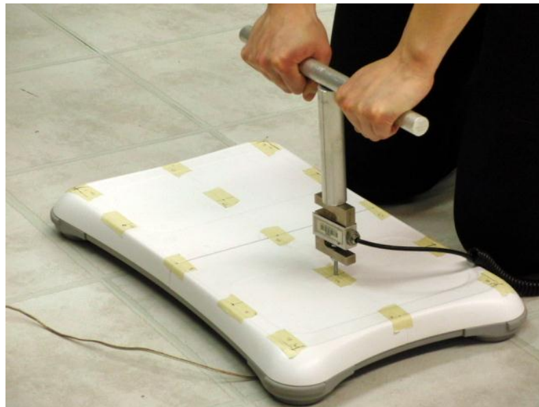
Figure 2-1: Equipment setup for COP accuracy testing. The Chatillon force transducer was custom fitted with a screw end and loaded with 20 kg of force at each of the 15 grid points.
