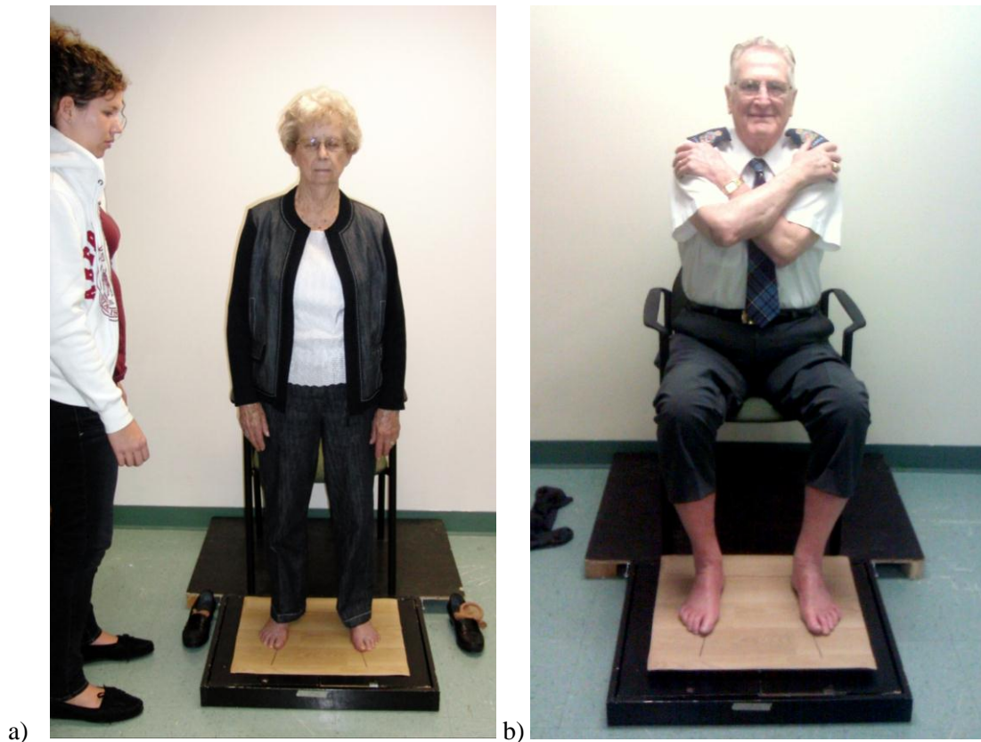
Figure 3-3: Set up of testing sessions for resilient rolled sheet condition during a) quiet stance and b) sit-to-stand tasks. The two Nintendo Wii Balance Boards are covered by a wooden platform, upon which the experimental floor samples are mounted (foreground).
