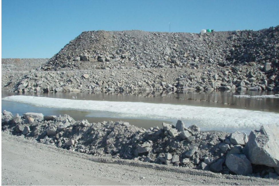
Figure 3-4: Type III test pile. Waste rock used in construction has similar average S content and exposure time as the drilling location at the Upper Type III waste rock dump.
