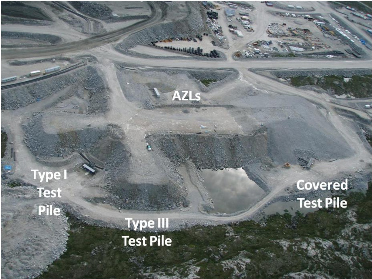
Figure 2-2: Test piles Waste Rock Research Site located at Diavik Diamond Mine.
