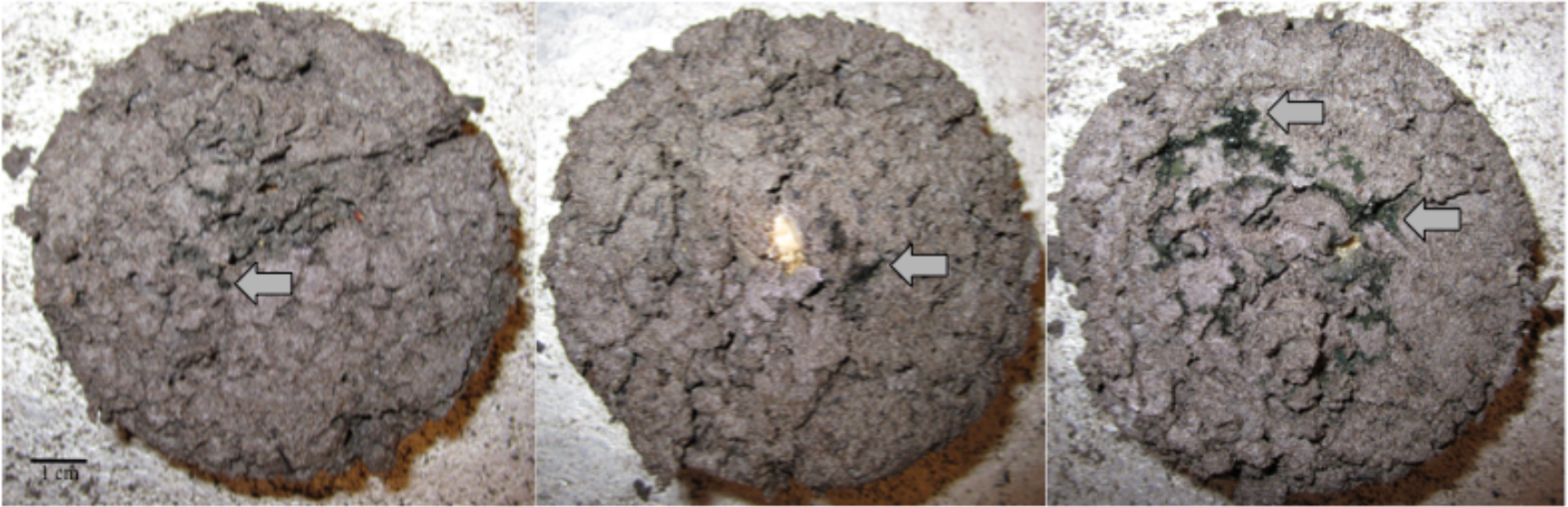
Fig. 3.1.2. Photographs of Eisenia andrei test soil from test units after the soil was removed and before adult removal. Image A is taken from test unit 560-4, B from 1000-1, and C from 1800-8. Note the black deposits (marked by arrows) seen in all three soil samples, with the most intense deposits found in C.
