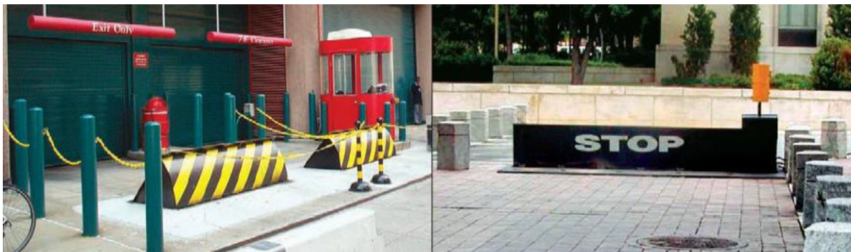
Figure 5: Road Blockers: note their ability to effectively bar auto traffic from an entire street with the push of a button. Source: FEMA 430
