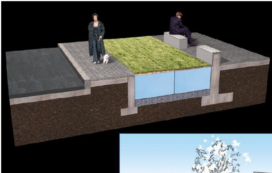
Figure 11: When installed tiger traps provide an invisible anti-vehicle trap which effectively immobilizes a vehicle and which does not interfere with pedestrian traffic or traffic flow on city streets Source: FEMA 430
