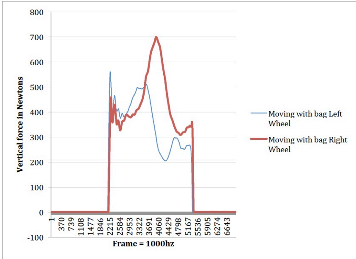
Figure 3.5.1, Graph of downward force on the front wheels of a Quickie GPV wheelchair. The graph illustrates the downward force and dispersal of weight over two wheels.
