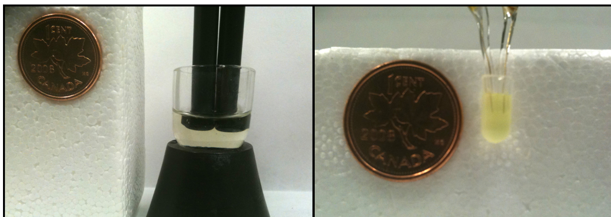
Figure 2.3: Comparison of standard-size gold disk electrodes (left) and the microelectrodes (right). Approximately 40 \mu L cell suspension is sufficient for each electrochemical measurement when these microelectrodes are used.
