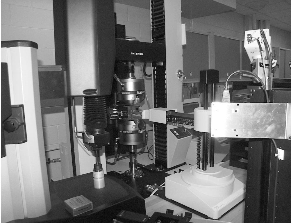
Figure 3.1: Automated tensile testing robot used at ALCAN KRDC.
