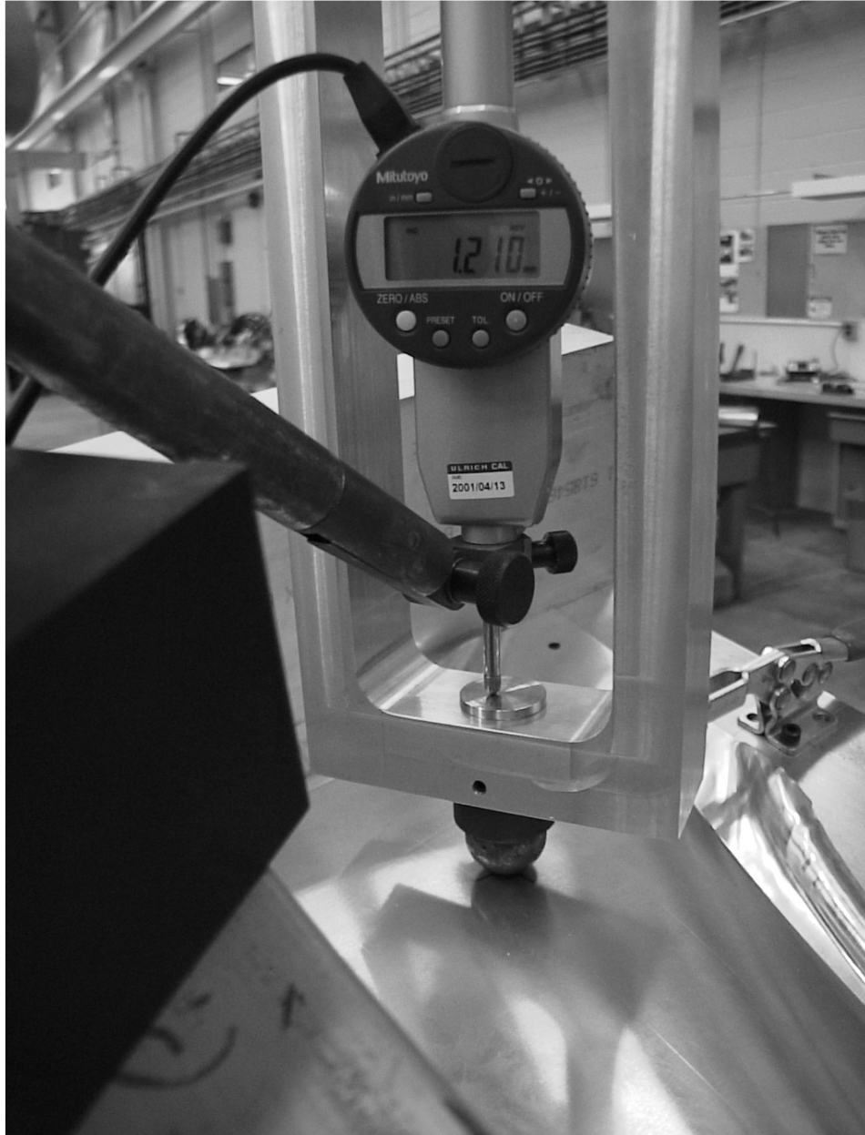
Figure 4.10: Close-up of the digital gauge used to measure normal displacement of the IRDI panel during static denting.
