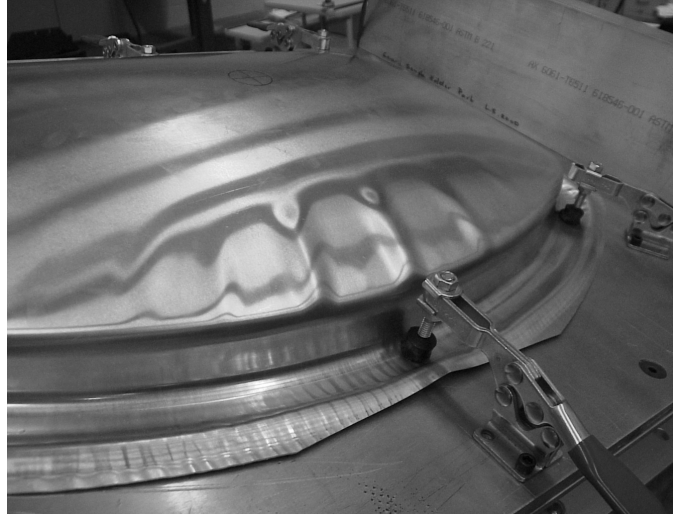
Figure 4.6: Wrinkles that were present in the 0.8mm and 0.93mm AA6111 sheet after forming.
