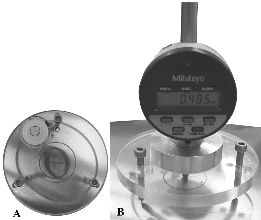
Figure 4.12: (a) Flat measuring platform that is positioned over the dent site, note the use of a bubble-type level to insure level positioning. (b) Measurement of panel location relative to the platform at the dent site.
