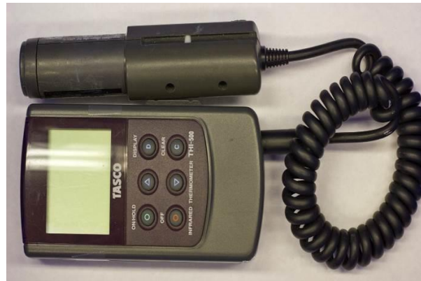
Figure 4-6: Tasco Thi-500 non- contact infrared thermometer used to measure surface temperatures
