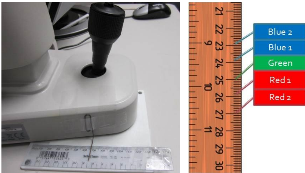
Figure 3-3: Setup for measuring distribution of RMS values in different degrees of defocus. Measurements were obtained when the pointer attached to the base were at 1 and 2 cm interval in both sides of green focus position using the scale attached next to the base.
