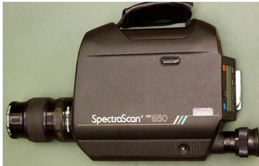
Figure 4-1: PR-650 SpectraScan photometer used to measure spectral characteristics of the Placido disc
