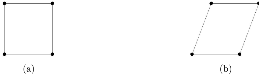
Figure 2.2: 2-D Schematic of Unit Micro-Structure of SMA in (a) Austenite and (b) Martensite Phases
