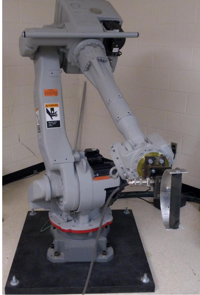
Figure 1: A force transducer was connected between a rigid D-Link handle and a MOTOMAP HP-50 robotic arm, allowing movement of the force transducer relative to the participant.
