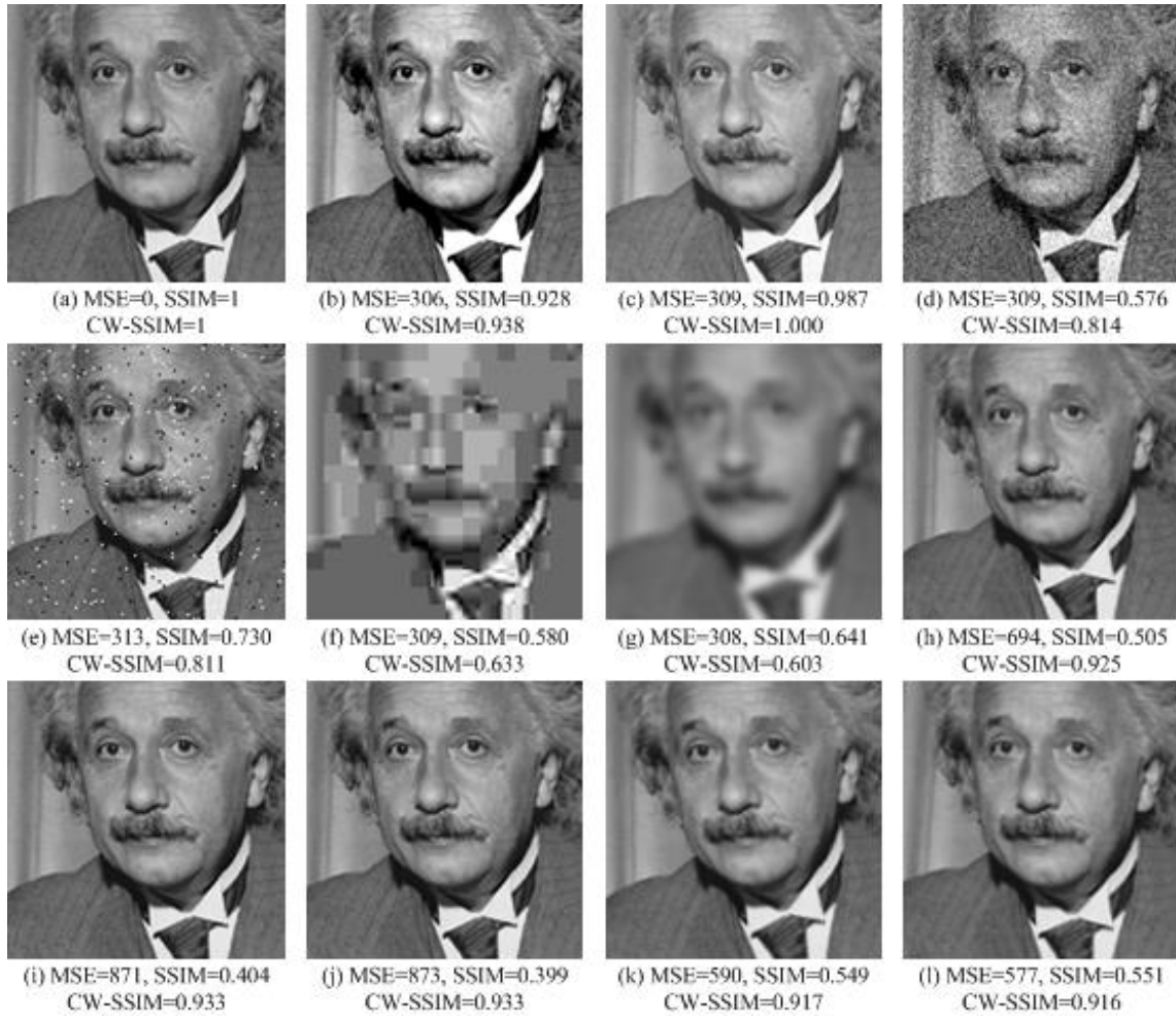
Figure 2.4: Comparison of image fidelity measures for “Einstein” image altered with different types of distortions. (a) Reference image. (b) Mean contrast stretch. (c) Luminance shift. (d) Gaussian noise contamination. (e) Impulsive noise contamination. (f) JPEG compression. (g) Blurring. (h) Spatial scaling (zooming out). (i) Spatial shift (to the right). (j) Spatial shift (to the left). (k) Rotation (counter-clockwise). (l) Rotation (clockwise). (Example taken from Wang et al.’s paper [14])
