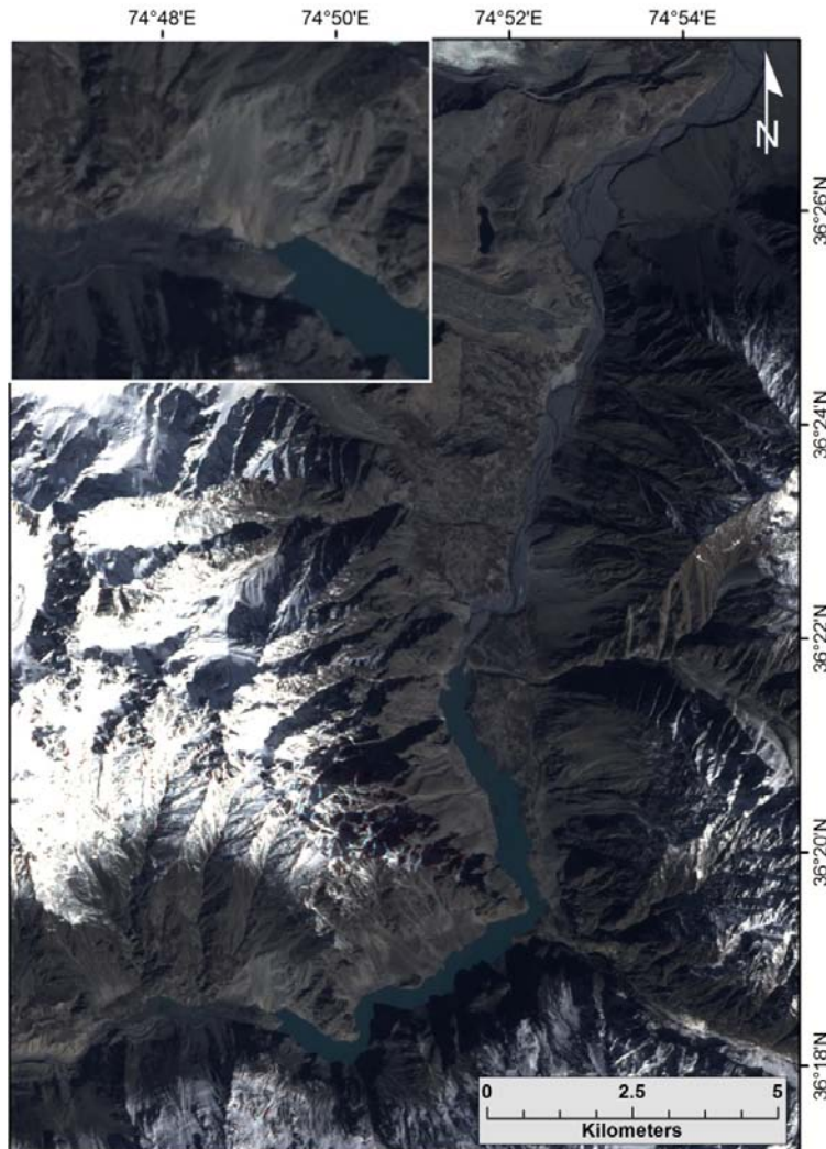
Figure 3.1: EO-1 satellite image obtained March 16th 2010 showing the Attabad rockslide and debris dam (inset) and the extent of rockslide-dammed Lake Gojal 72 days after impoundment.
