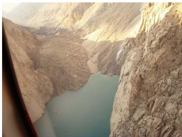
Figure 3.3: Aerial view of the Attabad rockslide (looking downstream) on January 17 2010 (day 13). Note characteristics of natural debris dam that blocked the Hunza River forming Lake Gojal, filling in lower foreground [photograph from The Pamir Times ].
