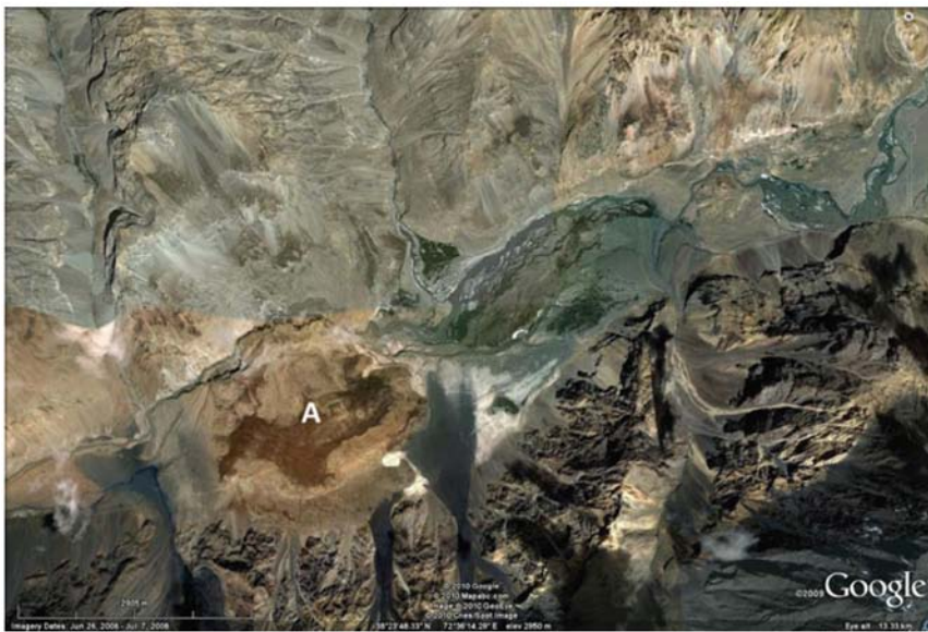
Figure 2.16: Google Earth image of the gigantic Pasor rockslide (A) that has blocked the Bartang River (flowing from right to left ) in the Pamirs of Tajikistan at 38^{\circ}23'03''\text{N} , 72^{\circ}34'49''\text{E} . The rockslide debris extends 2.72 km across the valley floor and has a volume in excess of 500 \text{ Mm}^3 .
