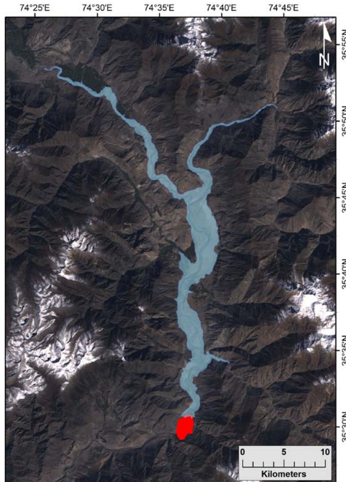
Figure 3.16: LANDSAT7 image with showing the 1841 rockslide debris dam on the Indus River and impoundment of the large reservoir downstream of Gilgit. The maximum pool elevation of the lake is estimated at 1,390 m a.s.l. Based on SRTM-3 data the 1841 rockslide-dammed lake had a maximum area of 88 km 2 and a volume of 6.5 Gm 3 (see Delaney and Evans, 2011).
