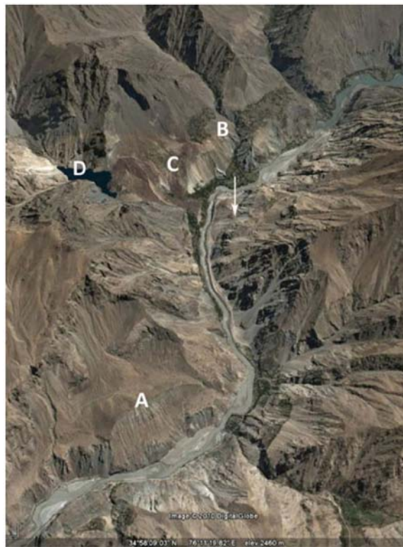
Figure 2.5: Typical example of complex valley fill deposits in the Upper Indus basin, northern Pakistan. Previously unmapped deposits include (1) older rockslide deposits at A and B that both dammed the Indus River, (2) younger rockslide deposits (C) that have dammed a tributary forming a rockslide-dammed lake at D and ran up the opposite valley side to a limit indicated by vertical arrow . This rockslide also dammed the Indus. Length of Indus (flowing from top right to bottom left ) seen in image is 13 km. Google Earth image at 34°58'09"N, 76°11'19"E, 65 km SW of Skardu. Locality is indicated in Fig. 2.3.
