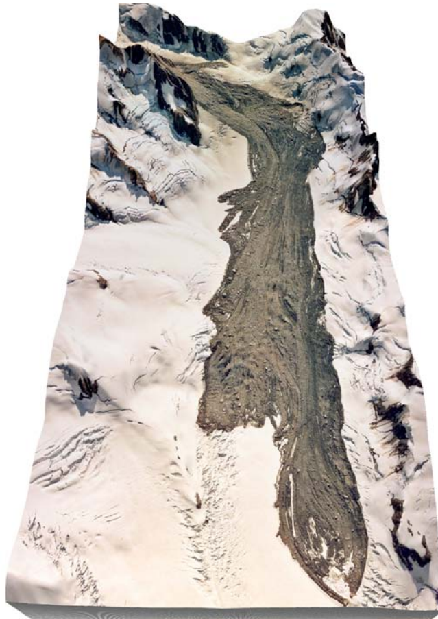
Figure 5.7: Perspective view to the southeast of the Mount Munday rock avalanche on Ice Valley Glacier, Waddington Range, southern Coast Mountains. Image prepared from orthorectified aerial photographs flown on August 20, 1997 draped over DEM prepared by photogrammetry from the same photographs. Note flow lines in debris.
