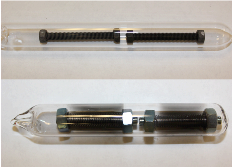
Figure 4-3. Picture of mandrels with stents sealed in a quartz tube after heat treatment. (a) Purchased mandrel and (b) Machined mandrel, showing contamination
